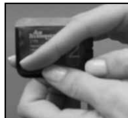
Figure 6c Seal the Barrier Envelope.
